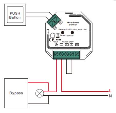
Note: Please follow the detailed wiring diagram of corresponding 2-wire dimmer or switch.
